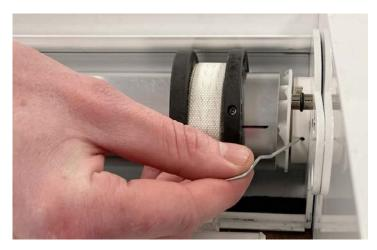
Press and hold the reset button (using a pin) till the blind shunts (moves) a couple of times. The motor is now activated and the blind is ready for pairing.
