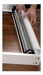
Remove the cover plate screw and carefully take off the cover plate.
