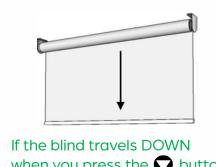
If the blind travels DOWN when you press the button you can skip the rest of this page and move straight on to setting the limits
