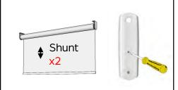
Press and hold the button on the back of the handset until the blind shunts 2 times with a pause between the shunts
