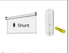
Press and hold the red button on the back of the remote until the motor shunts
